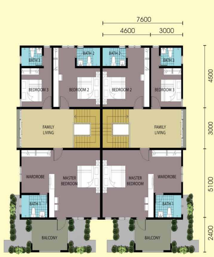
First Floor / 一楼平面图
